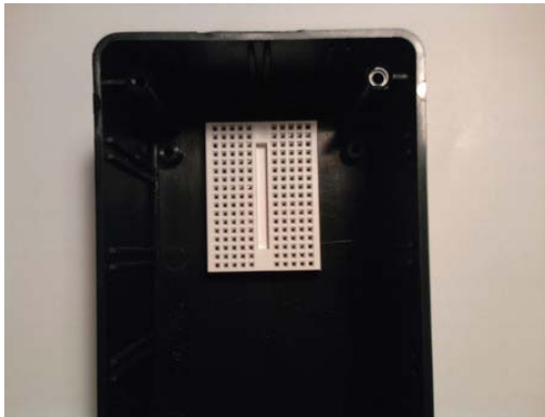
Figure 6-11. Add bread board to project
