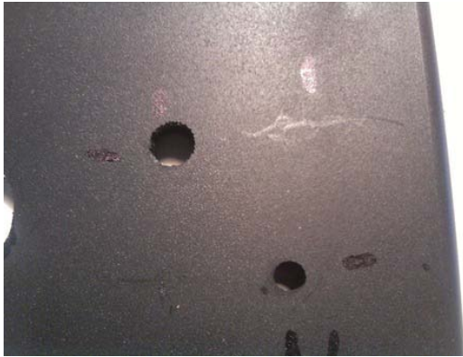
Figure 8-3. Drill holes for the ultrasonic bracket.
