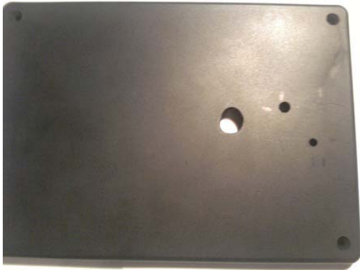
Figure 8-4. Drill a hole so the ultrasonic wires can be connected to solderless breadboard.
