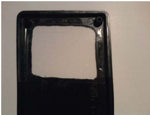
Figure 6-10. Clear screen attached with double-sided tape
