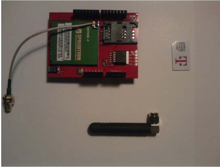
Figure 9-1. Cellular Shield with duck antenna and T-mobile SIM card
