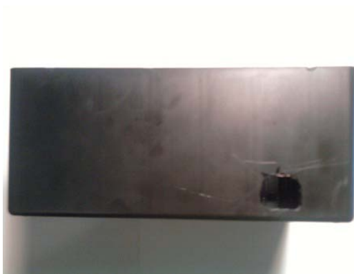
Figure 8-7. Drill a hole so that power can be connected to the Arduino.
