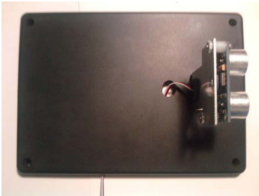
Figure 8-6. Attach ultrasonic sensor to bracket.
